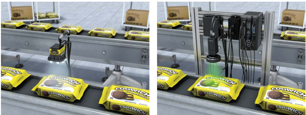
Figure 1: An example of an integrated smart camera and embedded controller system. Both have advantages in flexibility and development.
